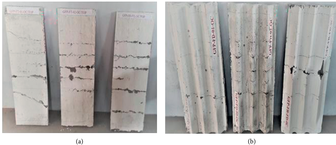
FIGURE 13: Cracking behavior of GF panels under flexure. (a) Flat panels. (b) Folded panels.
