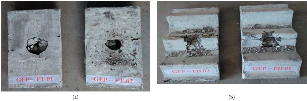
FIGURE 16: Cracking behavior of GF panels under impact. (a) GF flat panels. (b) GF folded panels.
