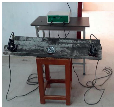
FIGURE 7: Ultrasonic pulse velocity test.
