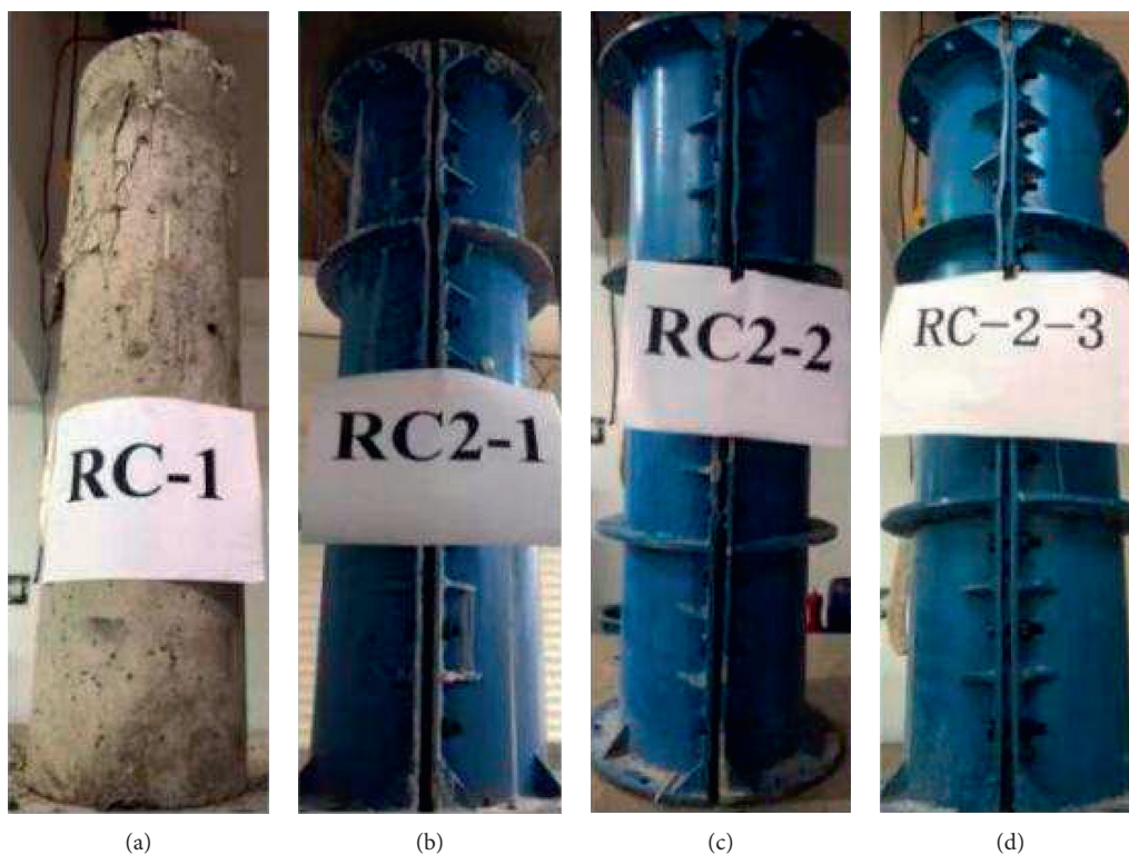
FIGURE 6: Failure modes of typical specimens.
