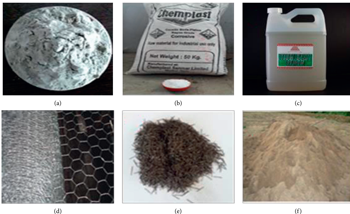
FIGURE 2: Constituents of geopolymer ferrocement. (a) Fly ash. (b) Sodium hydroxide. (c) Sodium silicate. (d) Wire mesh. (e) Steel fiber. (f) River sand.
