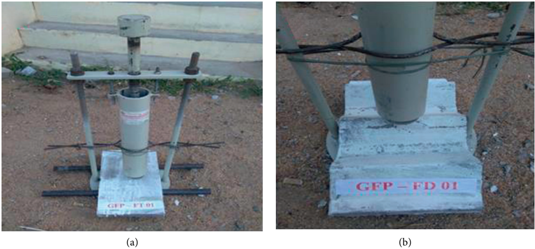
FIGURE 10: Drop-weight impact test on GF panels. (a) Test on flat panel. (b) Test on folded panel.
