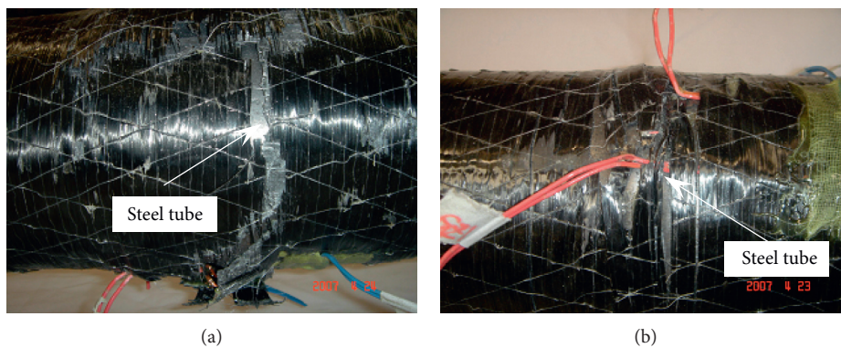
FIGURE 5: Fracture of CFRP of specimens with a small axial compression ratio. (a) Longitudinal CFRP of A1. (b) Transverse CFRP of A0.
