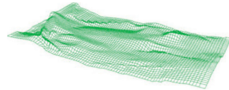
FIGURE 5: The mesh model of bottom plate of working face.
