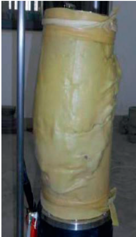
FIGURE 3: The specimen after the large-scale triaxial consolidated drained shear test.
