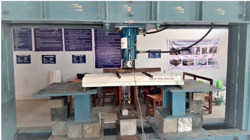
FIGURE 9: Flexural test on the GF folded panel.
