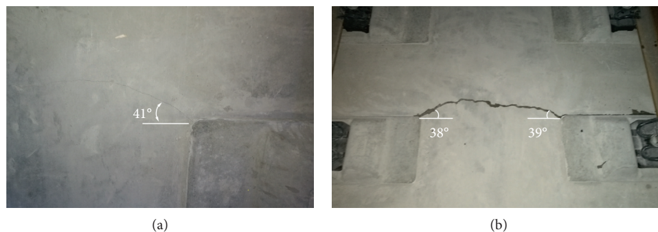
FIGURE 3: Distribution of cracks on the surface of track slab. (a) Initial crack. (b) Crack coalescence.
