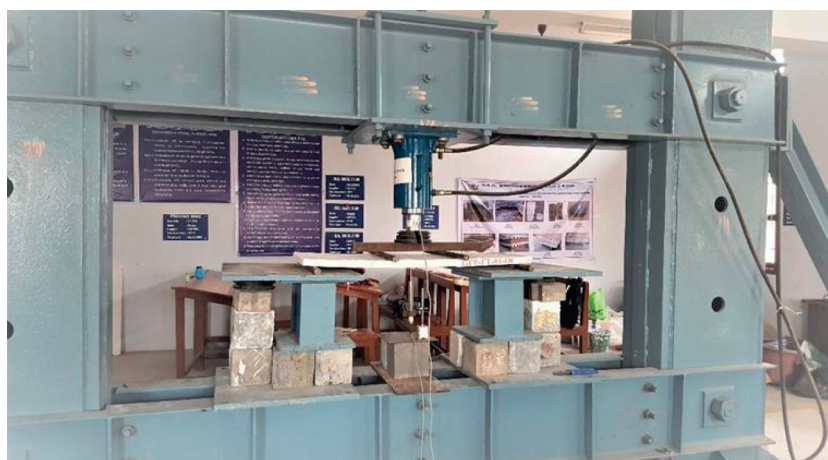
FIGURE 8: Flexural test on the GF flat panel.
