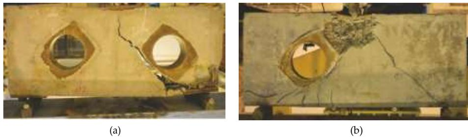
Figure 8: Failure modes of specimens strengthened with SPFs: (a) specimen *S-F* and (b) specimen *E-F*.
