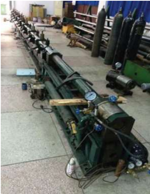
Figure 5: Components of the split Hopkinson pressure bar test system.
