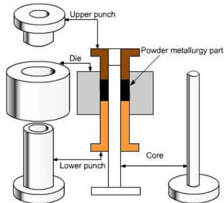
Figure 1: Parts of Die
