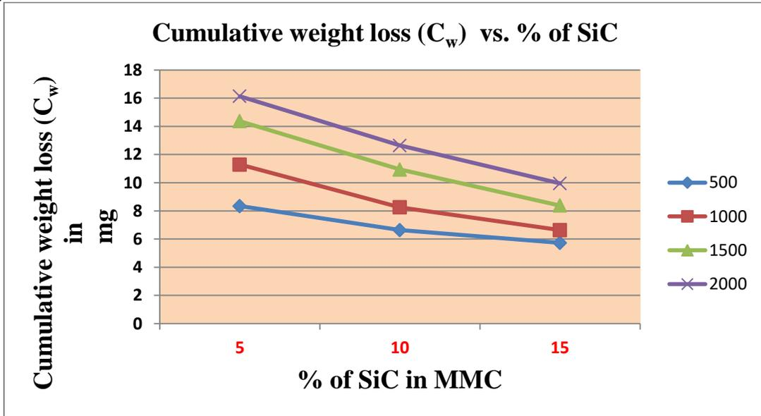
**Figure 13:** Graph of variation of Cumulative weight loss ( $C_w$ ) vs. % of SiC
