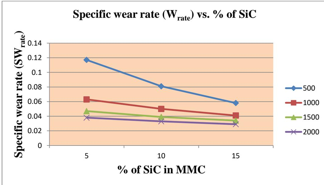
Figure 12: Graph of variation of Specific Wear rate (SW<sub>rate</sub>) vs. % of SiC
