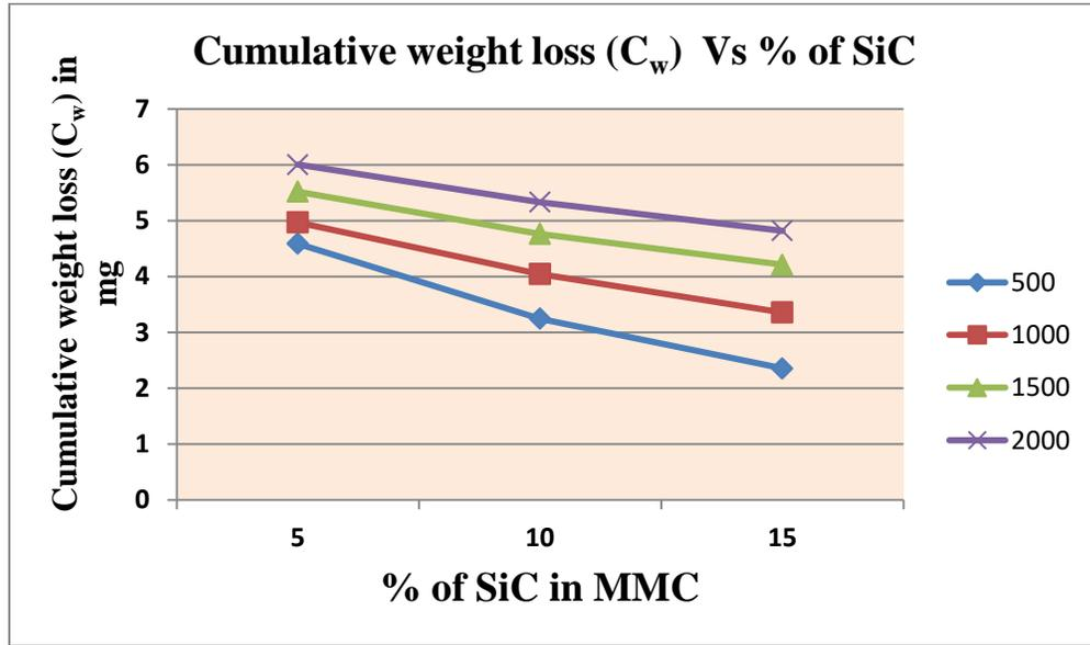
**Figure 9:** Graph of variation of cumulative weight loss ( $C_w$ ) vs. % of SiC
