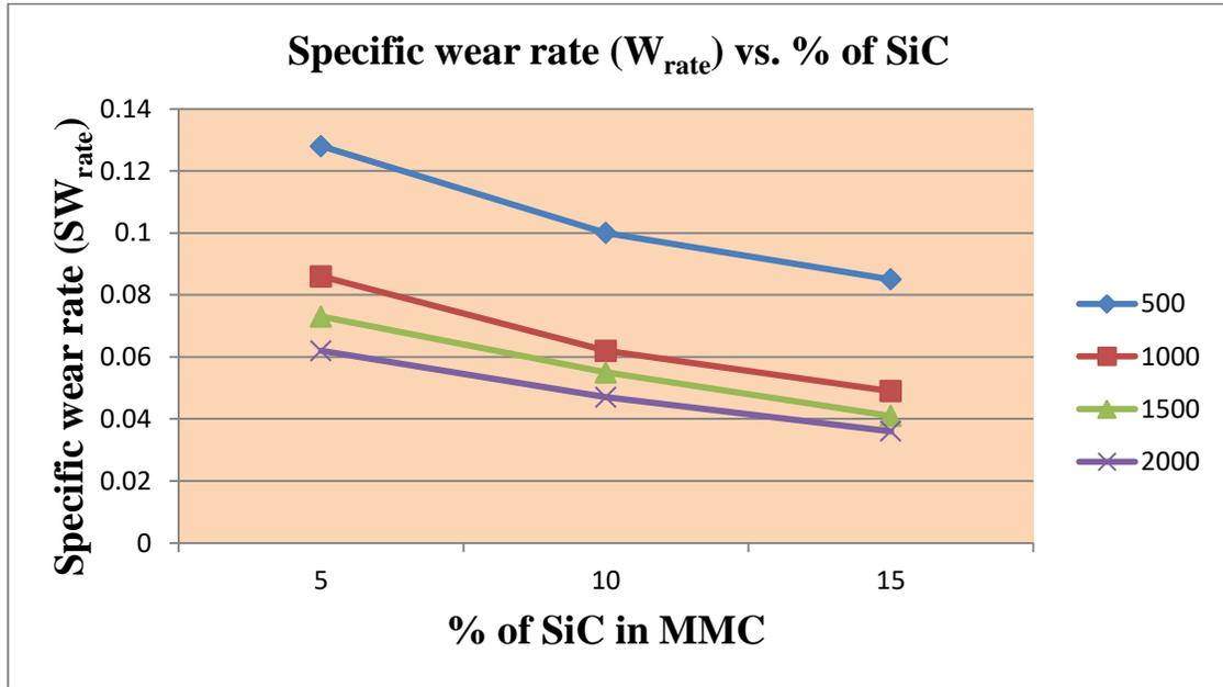
**Figure 16: Graph of variation of Specific Wear rate (SW<sub>rate</sub>) vs. % of SiC**
