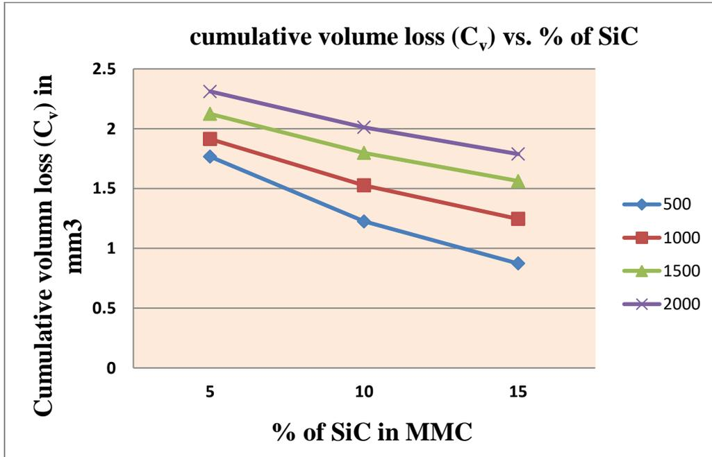
Figure 10: Graph of variation of cumulative volume loss (C<sub>v</sub>) vs. % of SiC
