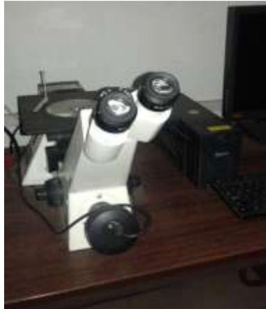
**Figure 5: Optical inverted microscope**
