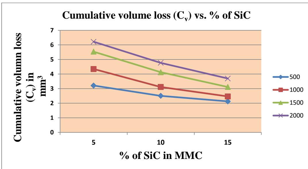
**Figure 14:** Graph of variation of Cumulative volume loss ( $C_v$ ) vs. % of SiC
