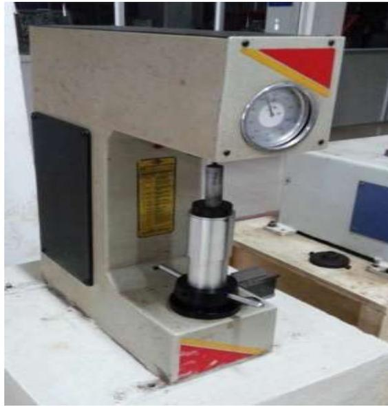
**Figure 7: Rockwell hardness tester**
