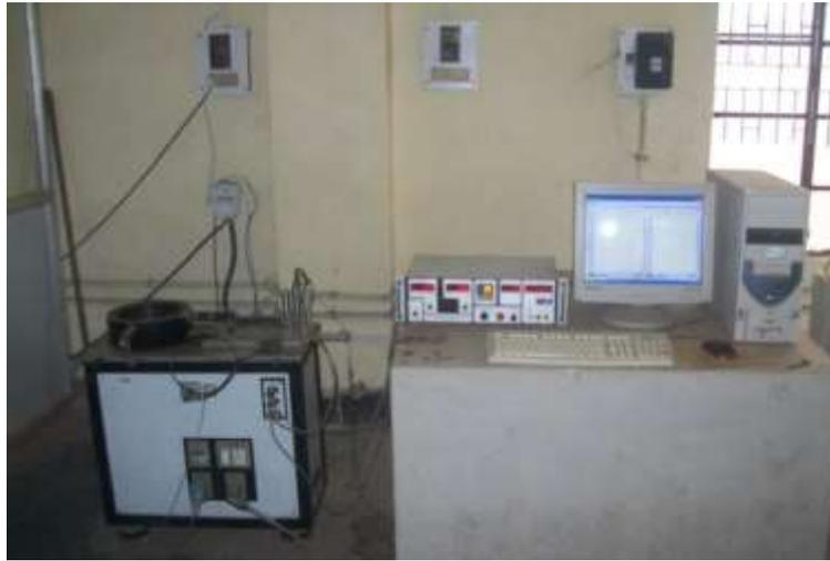
**Figure 4: Pin-on-disk apparatus for wear test**
