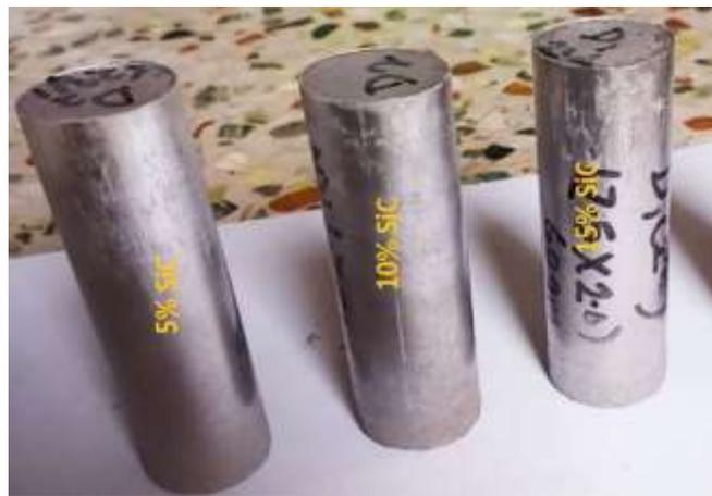
**Figure 3: Samples of AMMC produced with 5%, 10% and 15% SiC**
