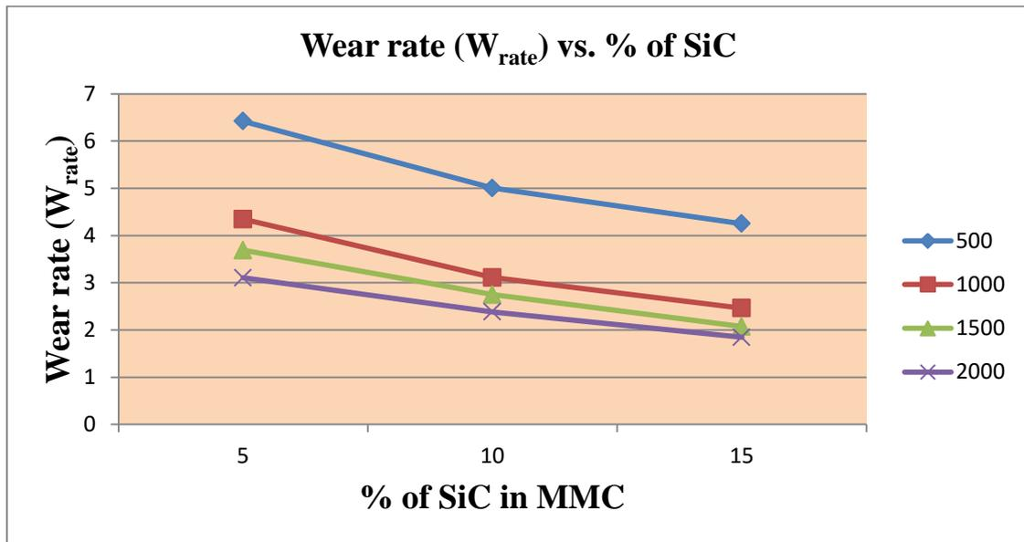
Figure 15: Graph of variation of Wear rate ( $SW_{rate}$ ) vs. % of SiC
