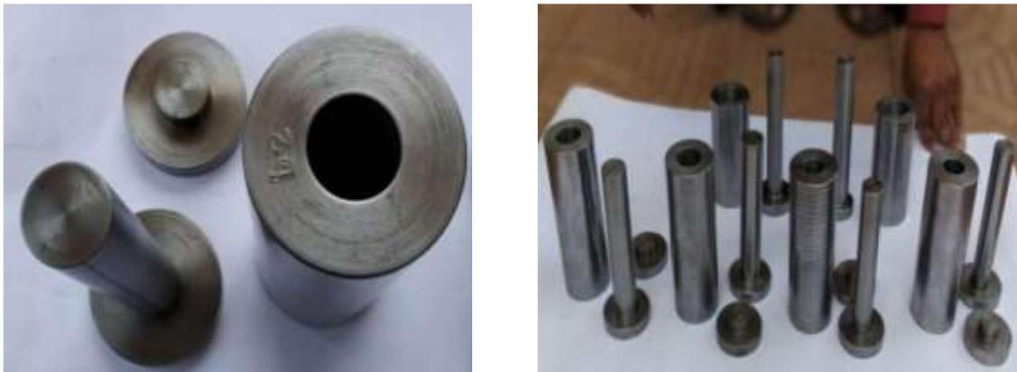
Figure 2: Die and punch system made of C45 steel.
