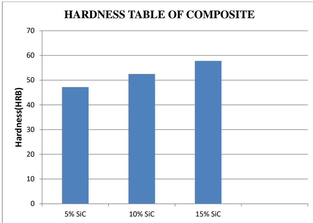
**Figure 8: Hardness of AMMC produced**
