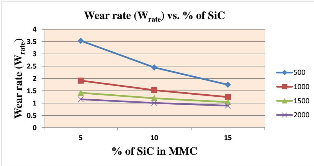
Figure 11: Graph of variation of Wear rate (W<sub>rate</sub>) vs. % of SiC
