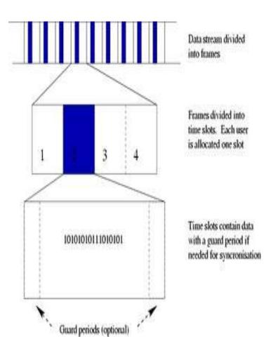
• Thus, in contrast to FDMA, the transmission inTDMA is discontinuous.
