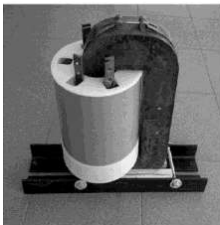
Fig.3. The model of the copper transformer Cu with a capacity of 10 kVA [16].
