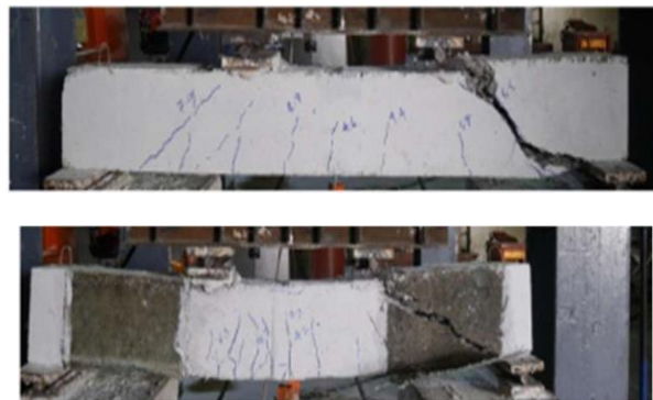
Figure 3. Failure modes of beams
