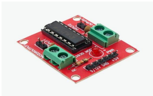
Fig.4 Proposed the motor driver(L293d)
